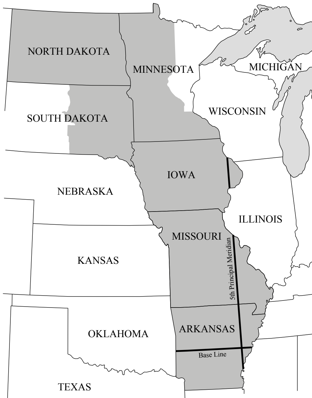
FIGURE 1 Lands Referenced to the Initial Point of the 5th Principal Meridian Taken from "Initial Points of the Rectangular Survey System" by Albert White (1996)
