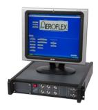
The IFF-45TS test set provides RF signal generation and parametric measurement of MK XIIA and TACAN equipment. Replies and interrogations can be individually configured to support testing requirements. ADS-B Out testing monitors ADS-B, TIS-B, ADS-R and acquisition squitters. The IFF-45TS emulates either a TACAN ground transponder or a TACAN airborne interrogator, providing six TACAN test modes.
