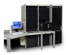
The RF Expansion Module (RFEM) is designed to support testing of airborne RF components on the ATEC® Series 6 ATE. Developed and manufactured by Cobham AvComm in partnership with Spherea Test & Services, the RFEM provides a convenient platform that is completely compatible with new and existing ATEC® Series 6 ATE systems. Our objective is to offer test coverage of RF products from all major OEMs
