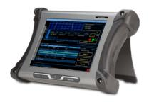
The ALT-8015 provides an easily configurable RF-based altitude simulation to quickly test an installation, or direct-connect to the Line Replaceable Unit (LRU) for additional troubleshooting capability. A large color touch-screen displays parametric measurements and allows for detailed profiles to be set up to emulate actual airborne conditions.
