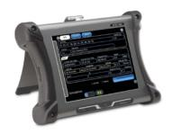
The GPSG-1000 uses modular technology for RF and baseband signal generation to produce highly accurate and repeatable test results. Unlike bench top simulators, Cobham AvComm's approach also allows the test system to be easily upgraded.
