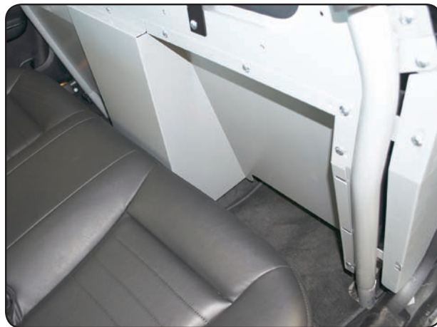
Picture from the rear seat of the new Charger. Design increases leg room so even larger prisoners can be transported easily.
