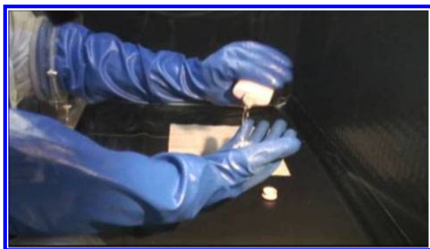
Figure 1 Pouring of powder into hands in glovebox.
