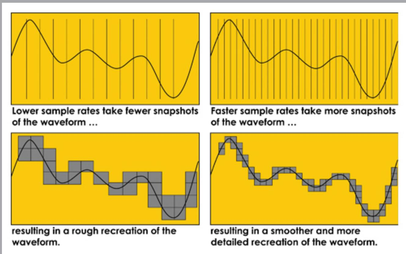
The higher the sampling rate, the better the resolution is in the reproduction of the original waveform (see simplified example, above), think more pixels in the picture on your TV set, and the higher the frequency the recording can reproduce. The greater the bit rate (bit depth), the greater the dynamic range potential of the recording will be. This is directly related to the signal to noise ratio of the recording; so for example, a 16 bit sample is capable of delivering about a 96dB S/N.
