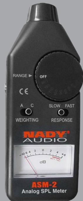
This analogue SPL meter's scale reads from minus dB through 0 dB to plus dB. On whatever scale you've set, when the needle points to 0 dB, the meter's reading that SPL level. For example, set to the 80 dB scale, the meter is reading 80 dB when the needle points to 0 dB.
