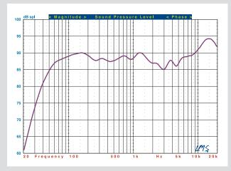
**Triton Five (purple**) +2.40/-3.46 dB, 200 Hz to 10 kHz; -3 dB @ 49 Hz, -6 dB @ 41 Hz; impedance minimum 4.35 ohms @ 3.9 kHz, phase angle -52.17° @ 2.9 kHz; sensitivity 88.5 dB, 500 Hz to 2 kHz.—*MJP*
