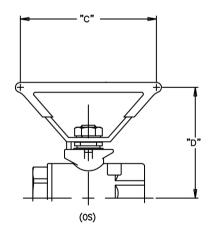
OS: The OS option provides clearance when a standard lever may interfere with adjacent piping or prevent accidental operation with a standard lever or other safety requirement.
