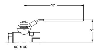
LL-SL: The LL and SL (spring loaded) option provides safety lockout of the handle in both the open and closed position. The SL option provides a spring loaded latch lock for situations when the valve is installed in a position where the locking feature would disengage. The spring loaded latch provides engagement of the lock in these positions without a padlock installed.
