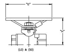
LO-SO: These optional handles provide the same features as the OS option but also offer the padlock and spring loaded lockout features.
