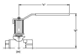
XH: The XH stem extension option provides clearance of the handle for operation when insulation on the piping system is required.
