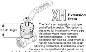
an ideal place for the "XH" stem extension. The external plastic shield helps to keep the insulation away from the stem extension, providing years of trouble free operation.
