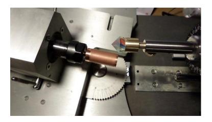
There are 9 round mandrels supplied with the machine, in copper, maple and phenolic and in 3 sizes.
