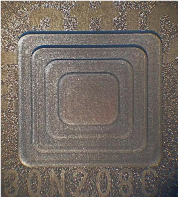
Figure 11: Optical verification after endpoint. Note the orange color in the bottom cavity reflected from the die.
