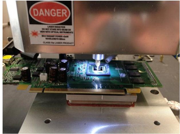
Figure 14: Graphics card mounted and electrically connected to floating endpoint sensor plate.
