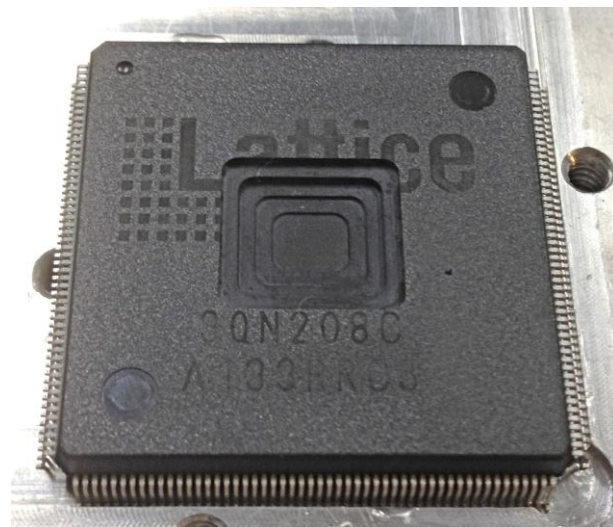
Figure 10: Step milling operation to endpoint resistively above the wire loops and capacitively over the die surface. No masking needed since the interior pocket was milled first. Target= 30 \mu\text{m} \pm 1 \mu\text{m} for the die and 5-10 \mu\text{m} above the wire loops.
