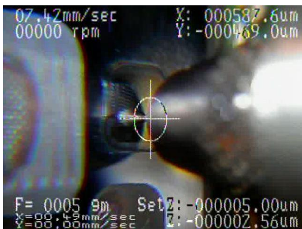
Figure 17: Soft carbon conductive tip touchdown and area scan to map remaining silicon thickness and identify minima. A 150 \mu\text{m} scan tip was used.
