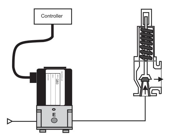
A Proportion-Air QB device is used to control the pressure of air to test the cracking pressure of a relief valve.
