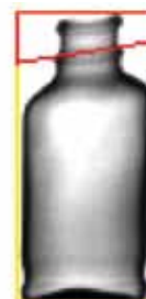
Figure 7: Detection of missing cap
