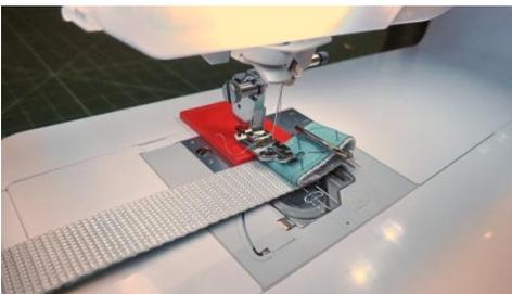
It goes behind the presser foot supporting the back of the sewing machine foot. Once you have your line of stitching started you can set it aside.
