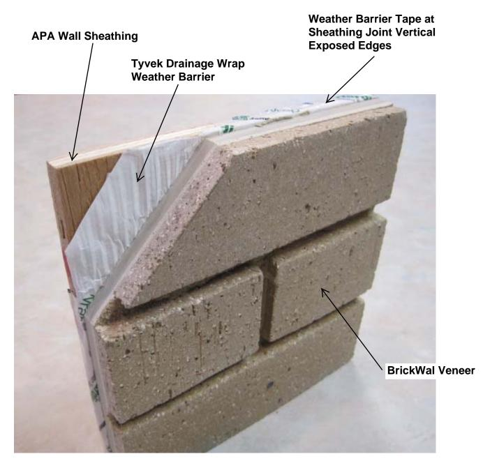
**Standard Detail With No Countinuous Insulation**
