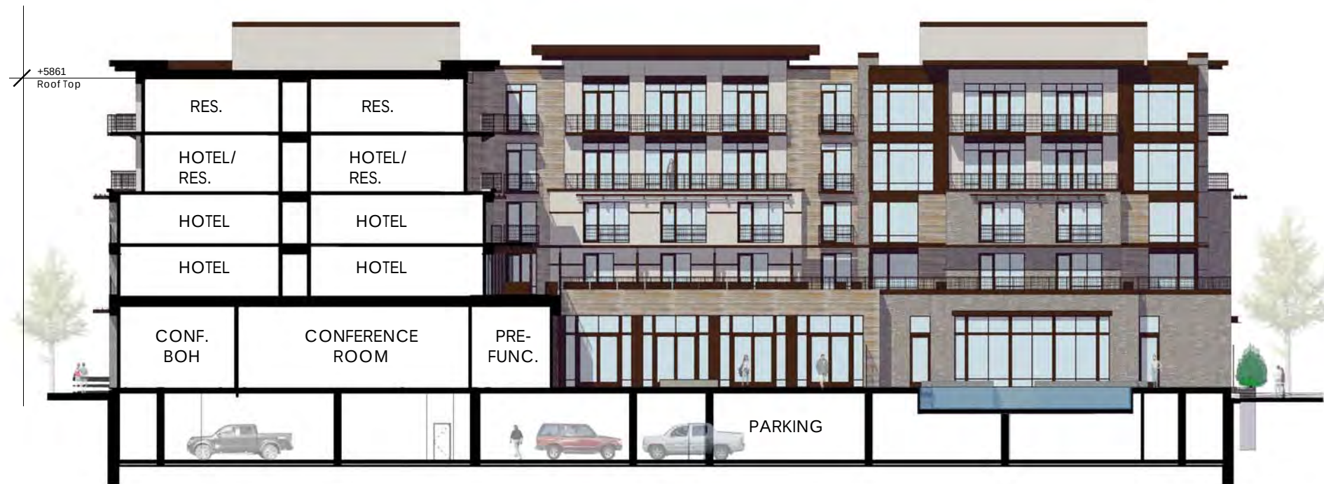
2 N/S BUILDING SECTION B-B SCALE 1" = 8'-0" 0' 8' 16' 32'
