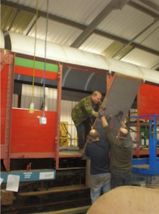
The side planking is trial-fitted and then removed section by section to allow the painting to top coat of the outer faces and edges. The sections are then reassembled on the van for the final time. New sidelight frames are being produced and fitted as well.
