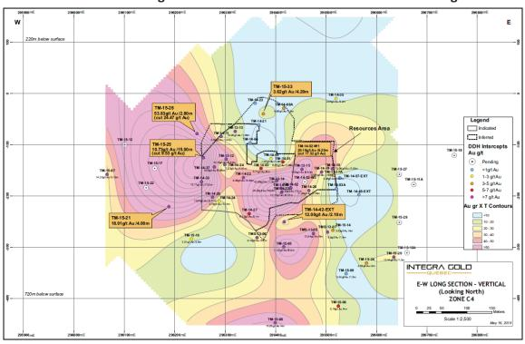
C4 Zone - Vertical Long Section with Grade X Thickness Contour Looking North
