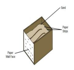
The objective of the GeoWall competition is to design and build a Mechanically Stabilized Earth (MSE) retaining wall model, using taped Kraft paper as reinforcements. The objective of the design is to use the least amount of reinforcement strips needed to support the retaining backfill and withstand loading phases.
