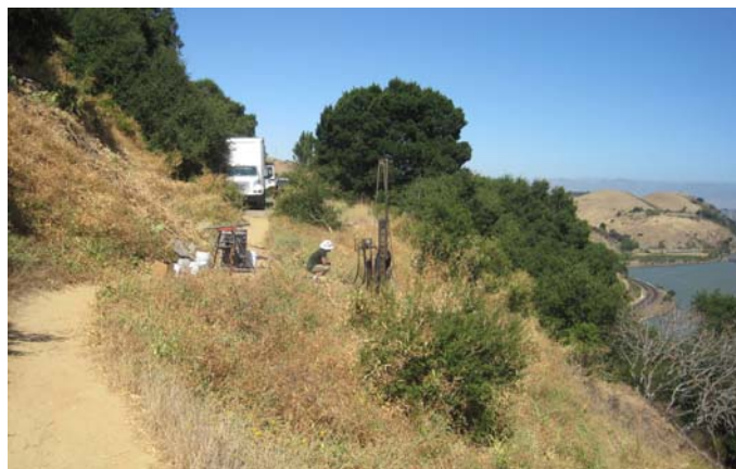
Figure 5. Portable hydraulic drilling rig situated on 1.25H:1V slope at large landslide at Station 176 (same view as Figure 9)
