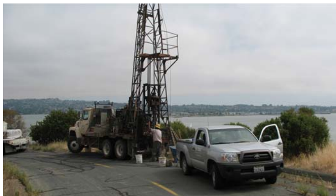
Figure 6. Truck-mounted drilling rig equipped with hollow stem augers
