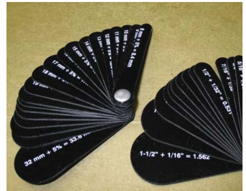
Correctly + 5% sized sheave gauges available from us.
