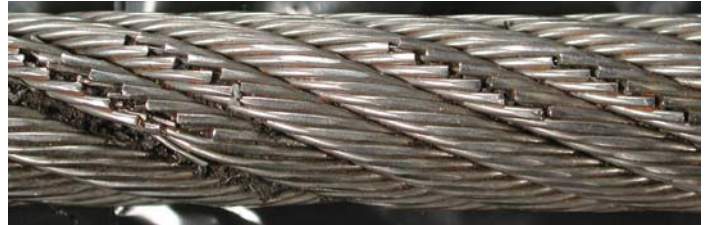
Example: Severe crown wire breaks on a 10-strand overhead crane wire rope. Crown breaks originate at the OUTSIDE of the rope at the contact point between rope and sheave/drum.
