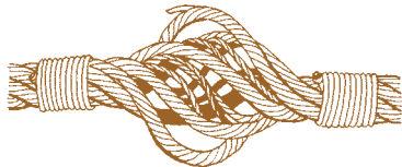
Bird Cage (6-strand rope) caused by shock loading.
