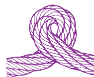
Kinked wire ropes which have been used. Kinks are pulled tight and caused distortion and failure.
