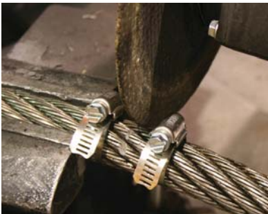
After attaching 3 hose clamps on either side of the cut mark, blade cut the rope.
