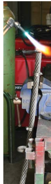
After blade cutting mount upright in a vice
