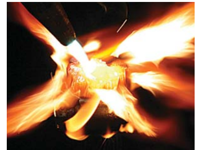
Carefully melt and fuse together all individual wires.
