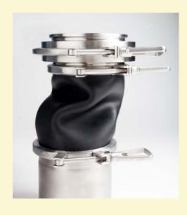
The CORA COMPENSATOR is a flexible sleeve that connects two pieces of machinery when rigid connections cannot be used due to vibration or off-axis. It can also be used in light overpressure/depression. The CORA COMPENSATOR is connected through a clamp band that can be opened easily when you need to sterilize the sleeve. It is also available with copper wire to ensure electrical conductivity.
