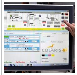
Windows<sup>®</sup>-based printing software with high-speed optical data transfer to the printing modules
