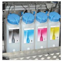
Open ink system with storage tanks of 10 lt. capacity, allowing refill without production stoppage
