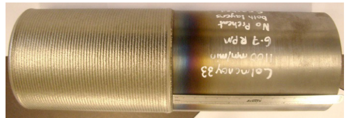
Colmonoy 133P2 Double Laser Clad Layer on Steel Roll
