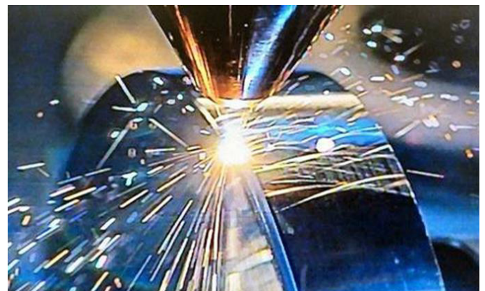
Wallex 40 being laser clad on a side trimmer knife in steel strip production
