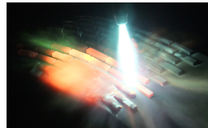
Figure 8: Colmonoy® 25F cementing tungsten carbide inserts onto an Integral Stabiliser for Oil & Gas Exploration Industry
