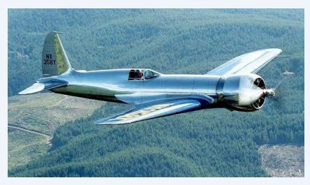
The aircraft was designed to reduce as much drag as possible. It had a polished aluminum exterior and was the first to feature a retractable landing gear with both main and tail wheel. It was the first to use flush rivets, split flaps and a special engine cowling built to reduce drag.
