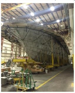
Yacht's hullform is a slightly smaller evolution of the 100 Motor Yacht's highly successful hull, incorporating similar tunnels to accommodate large propellers for improved performance and to reduce the draft.
