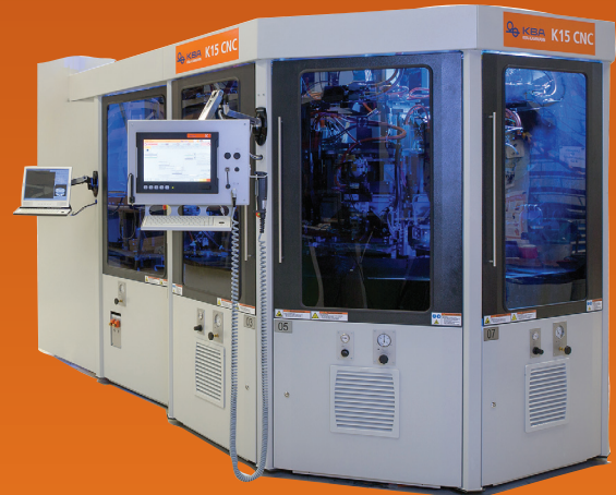
CNC Screen Technology Up to 6 colors on the Compact K15 CNC-S16
