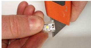
5. For end connection or jumping open one side of the connector and slide the end of the tape until it is flush with the back of the connector as shown. Close the connector top and snap in place. Make sure the (+) dot lines up with the red wire.
