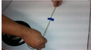
3. If Cutting is required, cut LED strip at cut points only, designated by the line between the corresponding pair of solder / connector dots.
