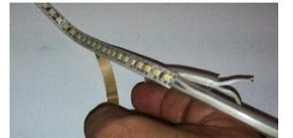
15. For outdoor rated (-P) material it is critical to adequately silicone all joints and cut points to prevent water damage. It is recommended to run silicone down the edge of the tape to provide further adhesion.
