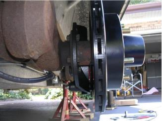
Notice the black plate mounted to the axel with six bolts. It carries the caliper with pads.
