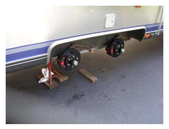
Hydraulic lines were bled and ready for tires. I did this in the spring of 2011 and replaced pads in 2013, overly concerned about scoring the discs. The parts were bought over the internet. Some parts are now locally available and even installation is available.
