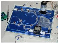
integrated heater maintained a system temperature of 37 degrees Celsius (98.6 F). Miniature heater modules were mounted at certain points along the "arterial path", used to simulate arterial "hot spots" the catheter had been designed to identify.
