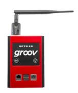
So even if there's no wireless network available, when you're close to the *groov* Box you can still connect your mobile device to *groov* and securely use the operator interface you've built.
