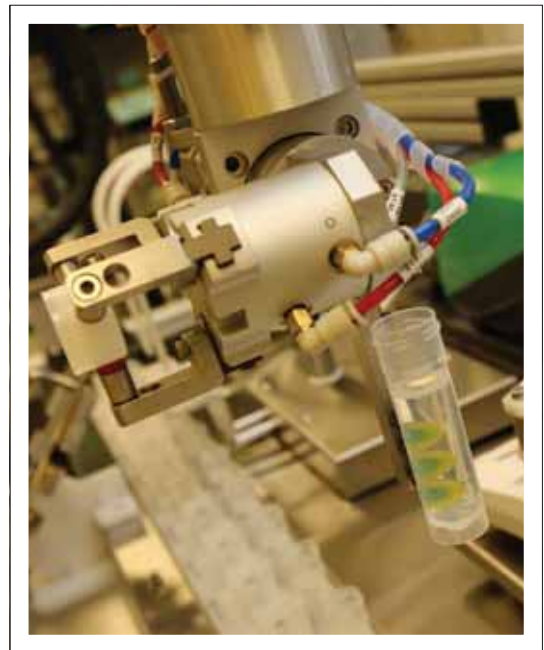
CAPPING/TIPPING ROBOT. In this photo, the robotic bottling system’s capping/tipping robot carries a filled vial to the scale to verify weight.
