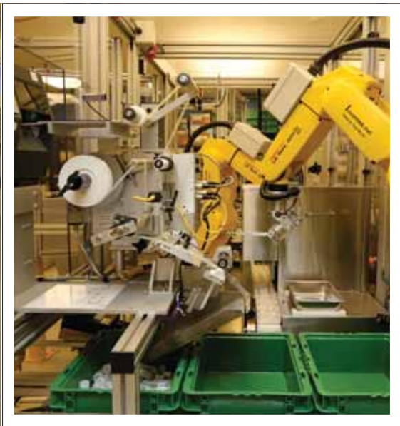
OFFLOAD ROBOT. The offload robot is visible in the middle of the screen with the label applicator to its left. At far left is the printer. Also shown at top left and bottom right are two vision system cameras that inspect labels exiting the printer and after they're applied to a vial.
