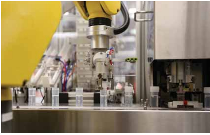
CAPPER ROBOT. This photo shows the capper robot of the robotic bottling system. To the right, a cap is torqued to the required specification by the torque servo.
