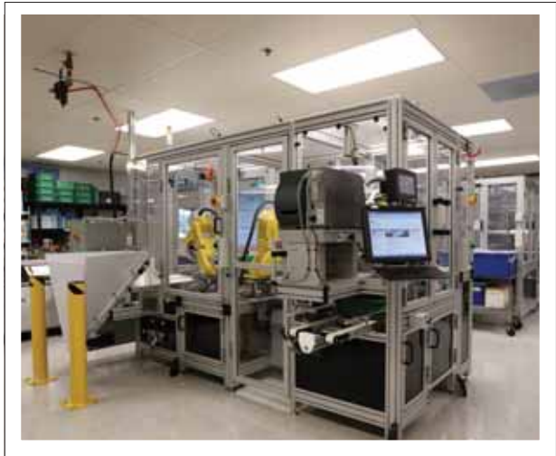
REAR VIEW. Shown in this view of the robotic bottling system is a secondary control display and a vision system display, as well as the back of the printer with offload conveyor, and a hopper that feeds empty bottles onto a light table.
