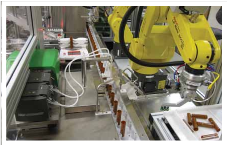
CONVEYOR LINE. Looking at the bottle load end of the system, the vision light table is seen in the lower right corner. It’s from this light table that the first robot picks up empty bottles, starting the process.
