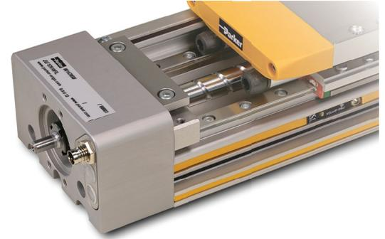
HMR ball screw driven actuators are designed for applications requiring high thrusts or higher precision. The ball screw driven version of the HMR offers 2 different lead profiles per frame size in order to maximize optimization of the drive train based upon throughput needs.
