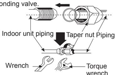
NOTE: First connect the pipe to indoor unit, then to outdoor unit. Be careful when bending pipe. Do not damage the connection pipe. Do not overtighten the nut or it may cause leakage.
