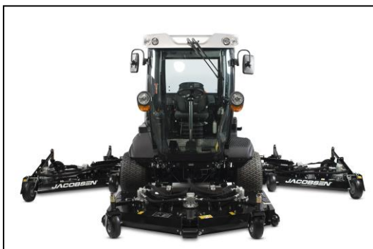
The Jacobsen HR800™ provides a cutting capacity of 100+ acres per day.
