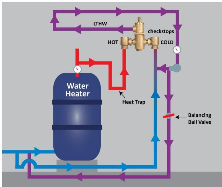
Figure 4 – A thermostatic mixing valve in a plumbing system
