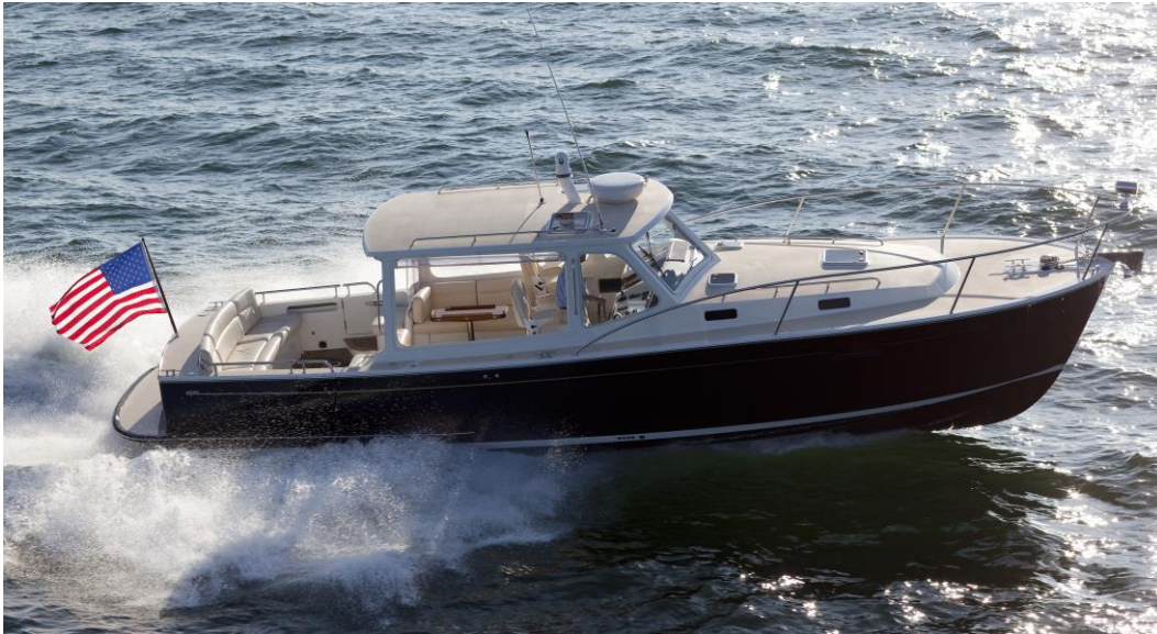
The MJM 36z underway powered with twin 220 HP sterndrive Volvo Penta D3s
