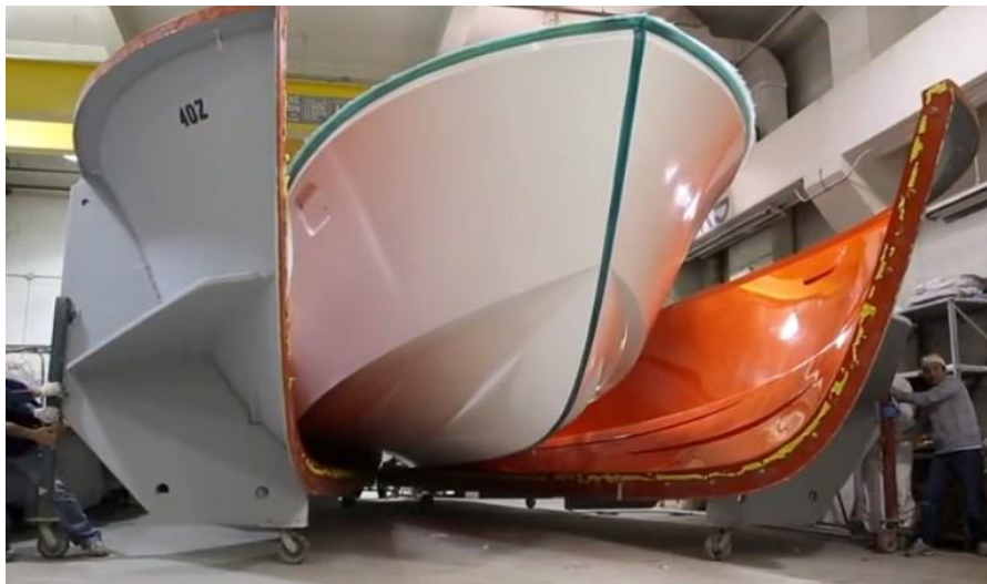
A 40z hull being removed from the molds after the oven post-cure process.
