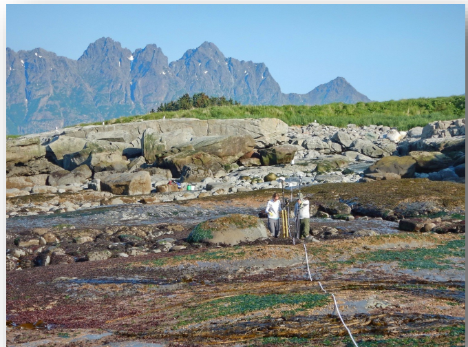
Mobile GPS units mapping detailed tidal elevation and position data. Photo by Mandy Lindeberg
