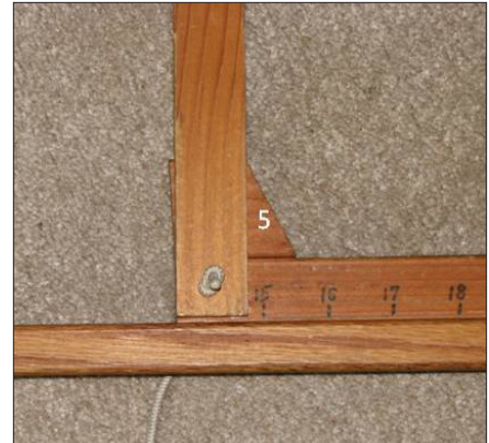
Figure 6. Triangle-shaped reinforcement piece (section 5) on the left jaw.
