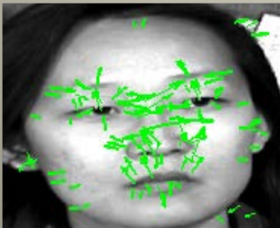
Keypoint selection with original SIFT method, 120 points
